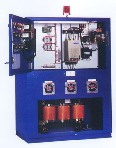
Spang Power Electronics designed and manufactured seven 50 KVA silicon carbide power supplies for Lindberg/MPH in Riverside, Ml. Each system consists of six (6) phase-angle fired SCR power controllers and a three phase transformer with six (6) secondary taps for precise load matching. These systems precisely control power to silicon carbide elements and maximize its useful life.
