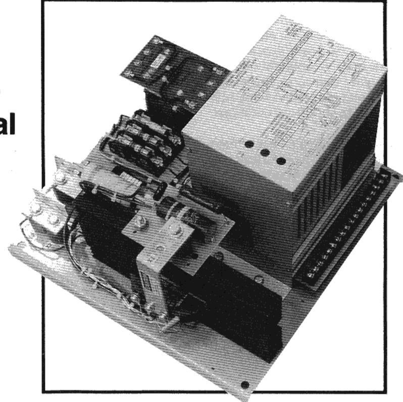
SPANG Power Control Units for single phase applications are available either with phase angle control or with synchronous firing control of the SCRs. Synchronous firing PCUs are normally applied to control static loads, such as resistive heating elements (nichrome), which are not affected by age or drastic change in resistance versus temperature.
