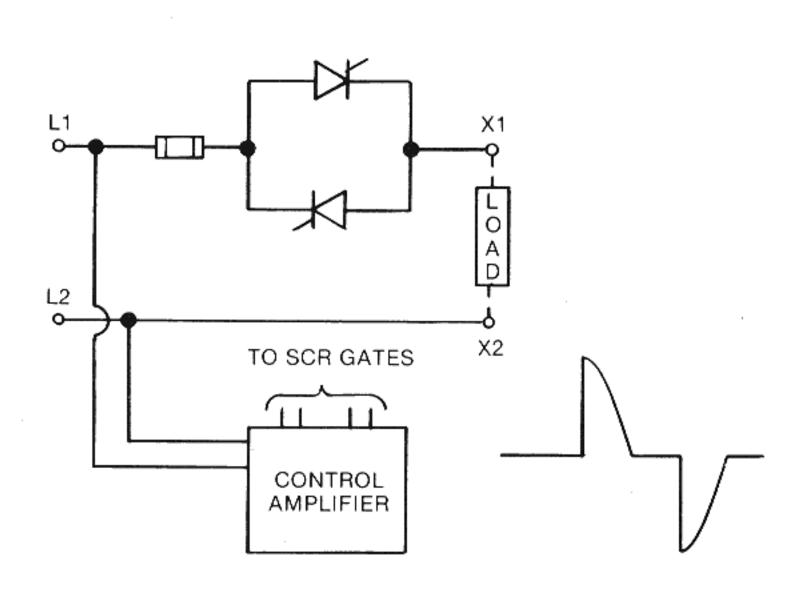
Fig. 1 Single Phase Converter & Waveform
