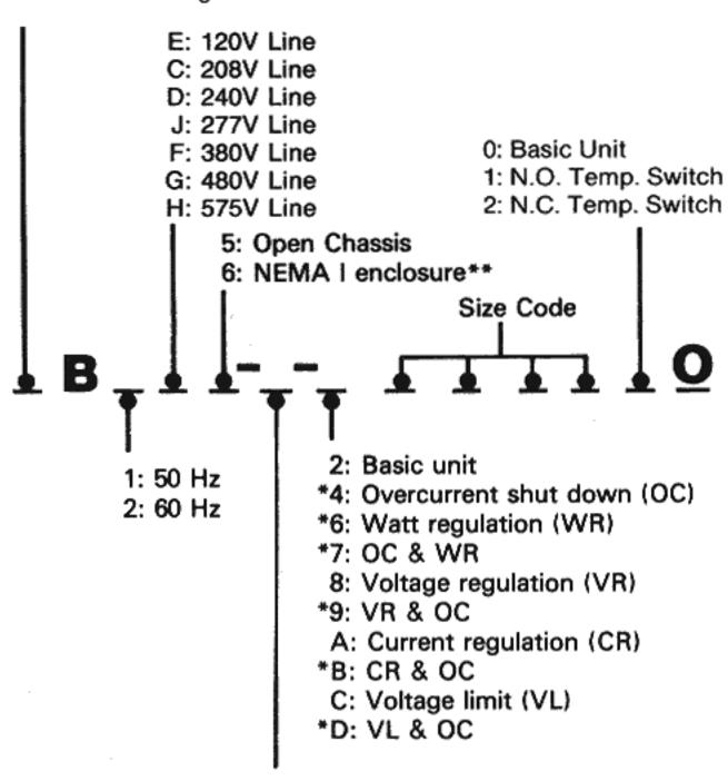
\*PCUs with these options must be tailored to individual requirements; consult factory before ordering. An additional 8" is required in height dimension for both chassis and NEMA 1 enclosures.
