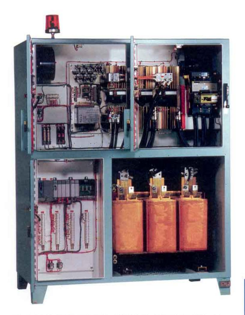
Spang Power Electronics designed and manufactured a single zone rectifier for electrophoretic paint deposition for Honda Motor Corporation of Mexico. This rectifier can supply 800 ADC at 400 VDC. It is being used in an indexing batch type system.
