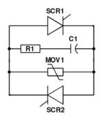
The typical failure mode of the circuit is the explosion of the MOV. MOVs
